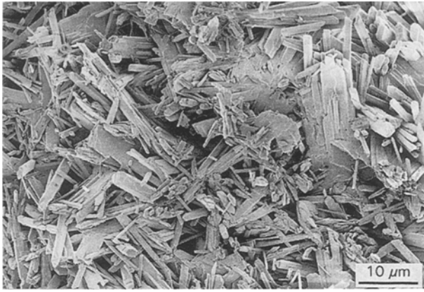
Figure 2 Typical aspect of a set plaster (65 vol % porosity) observed by scanning electron microscopy.
